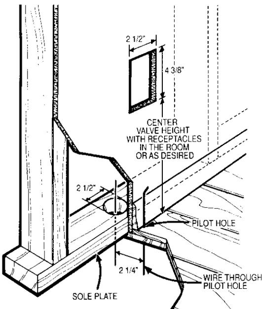
Having determined the location is suitable cut a 2 1/2" X 4 3/8" hole in the wall at the desired inlet valve location. Remove the side
