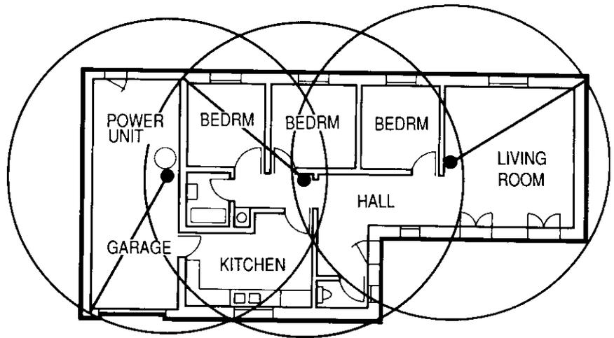
string or the hose itself can be used to help plan the layout. If working with 1/4' scale blueprints a seven-inch string can be used to represent the hose. If an electrical beater brush is to be used at present or in the future the inlet valve should be located within five feet of an electrical outlet. Air-turbine driven beater brush heads do not require electricity and thus allow more flexibility when choosing inlet valve locations.
