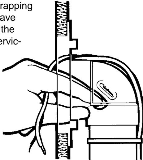
required due to overhead space restrictions. Precut these pieces and work quickly to prevent the cement on the end of the tubing from drying before it reaches the fitting at the valve below.
