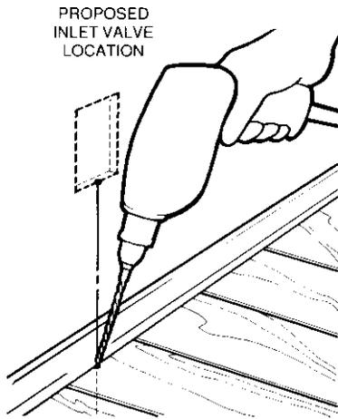
pilot hole through the floor and sub floor. The straight section of a wire coat hanger cut at an angle makes a good pilot hole drill bit. (Be careful not to snag carpeting.)
