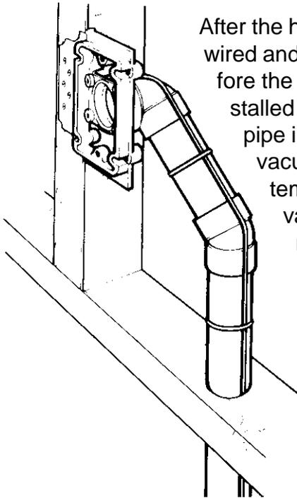
After the house has been wired and plumbed, but before the dry wall is installed is the best time to pipe in a central vacuum tubing system. Locate the inlet valve locations and nail the mounting plate to the nearest stud. Make sure the middle of the mounting
