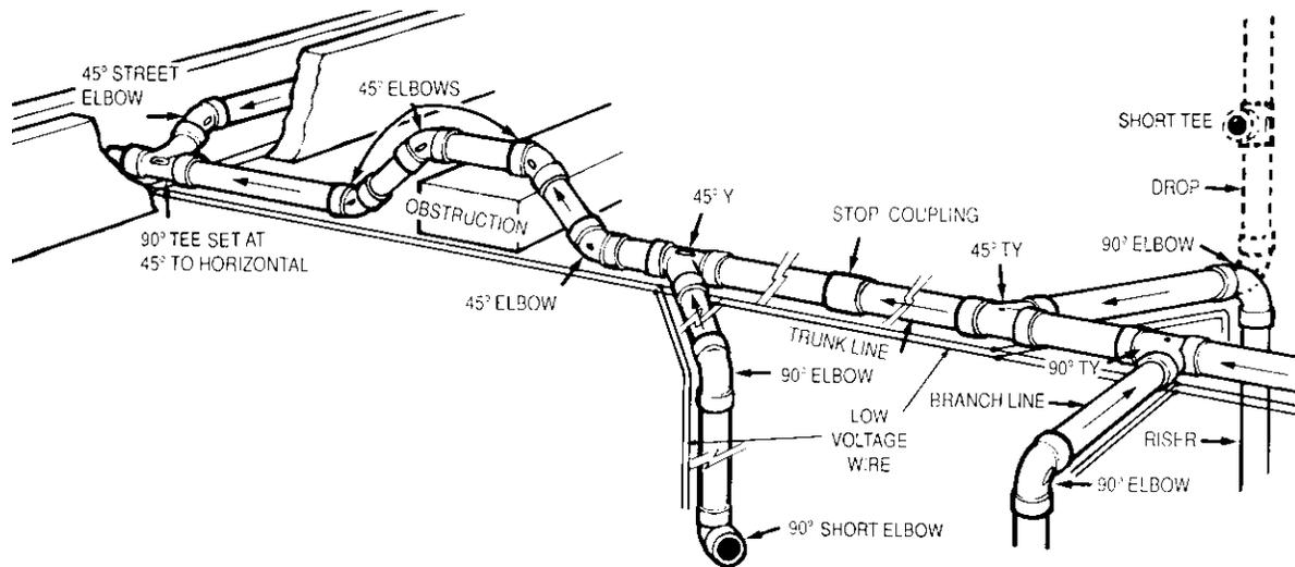
The amount of airflow that reaches the hose is dependent on the efficiency of the layout of the tubing system. Lines are to be kept as straight as possible. Tight 90 degree fittings are to be used only at inlet valve locations and sweep 90's used in all other applications.
